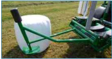
By means of the sidetip the machine automatically unloads the bale on the side. The flat sides of the wrapped bale have multiple film layers, so damage should be prevented by a hard stubble.
