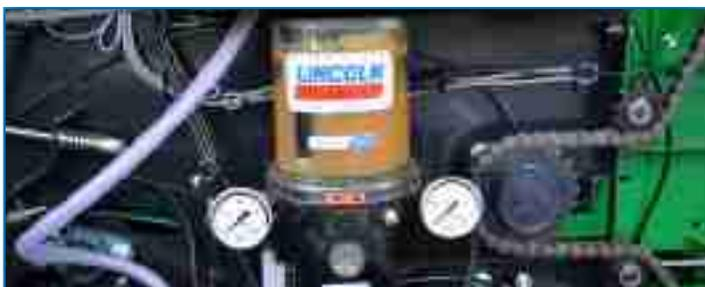
Lincoln auto greasing system. Simply and effective greasing of all bearings and rotating parts on the machine. Full automatic, 4 liter reservoir.
